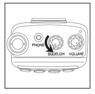
This action lowers the "squelch gate," allowing all signals and noise to get through.
